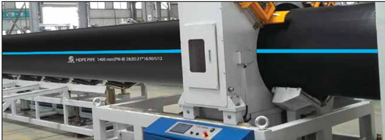
1400 mm RFL HDPE Pipe Production
